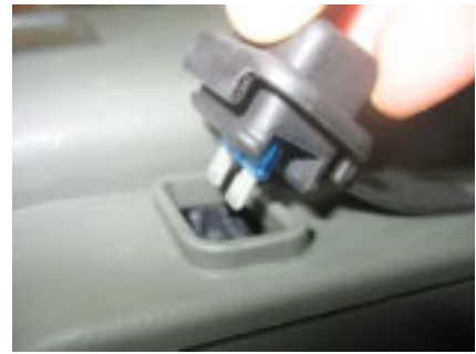
Figure 1.27 - Inserting batteries fuse
