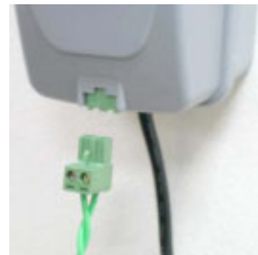
Figure 1.41 Plug the plot connector into the Perimeter Switch
