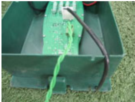
Figure 1.21 - Routing the Power Supply cord out of the cover
