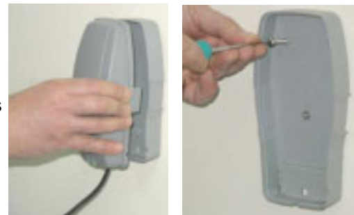
Mounting the Perimeter Switch using three mounting bosses on back cover
