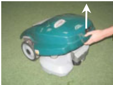
Figure 1.25 - Lifting the Bumper Cover
