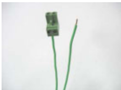
Figure 1.16 - Two loose wire ends at the starting point
