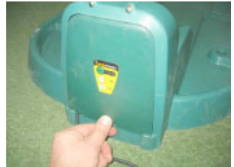
Figure 1.22 - Closing the Base Station cover
