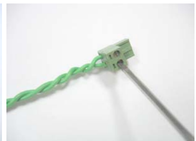
Figure 1.18 - Tighten the screw to secure the perimeter wire into the connector
