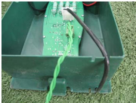
Figure 1.21 - Routing the Power Supply cord out of the cover
