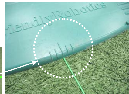
Figure 1.23 - Base Station alignment
