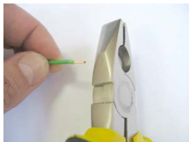
Figure 1.17 - Strip 6mm of insulation from the wire end
