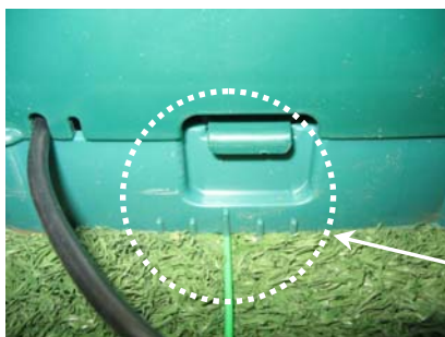
Figure 1.23 - Base Station alignment
